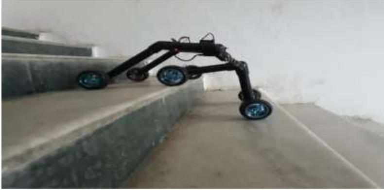
Fig. 5: rocker bogie climbing stairs
