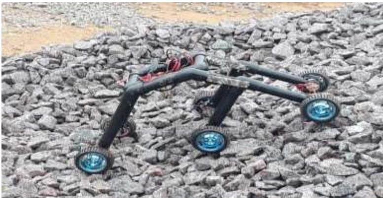
Fig. 4: Rocker bogie at uneven surface
